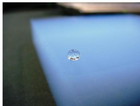
Fig. 1. Water drop on hydrophobic (water-resistant) aerogel (ID=LGG3-4b,  $n = 1.009$ ).
