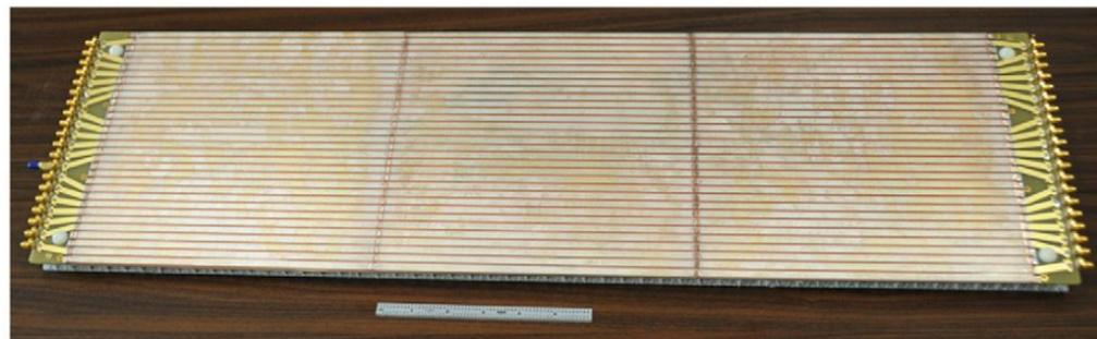
Three 20×20 cm<sup>2</sup> readout board chained
