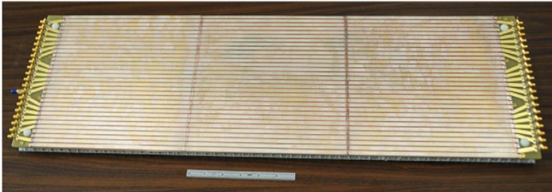
Figure 13. The 3-tile anode, a total coverage of  $20 \times 60 \text{ cm}^2$ . The connections between anode strips on neighboring tiles have been made by soldering small strips of copper to the silver silk-screened strips on the glass [19].
