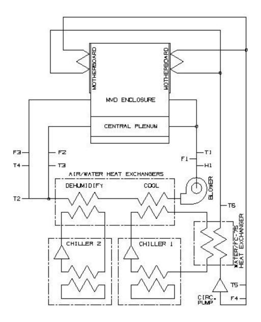
Figure 2: MVD Heat Exchanger Assembly
