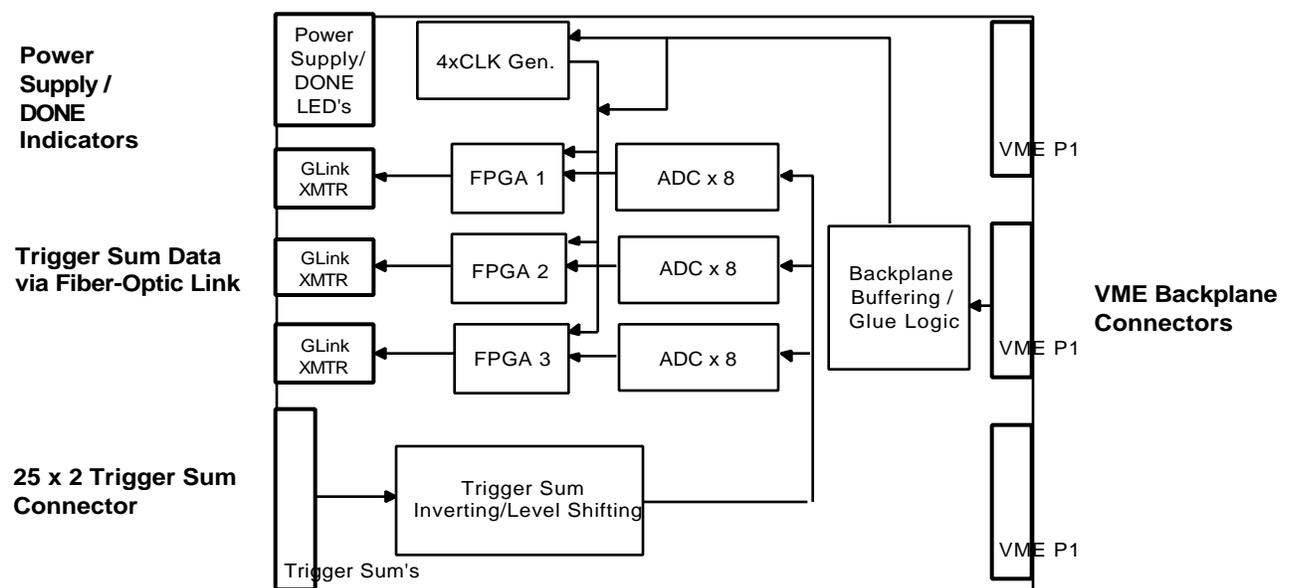
Figure 4. TIM Physical Layout and Connector Location
