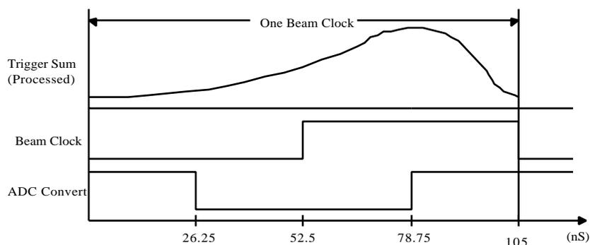
Figure 2. TIM Input Signal Processing and Conversion Timing
