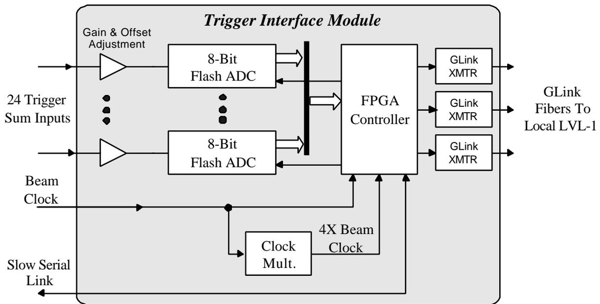
Figure 1. Trigger Interface Module Block Diagram
