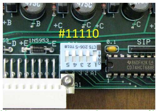
Module addresses are set on DIP switch near center of back edge of board A1 = bit0, A2 = bit1 ... A5 = bit 4
