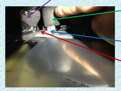
Shown are the Strip Pixel lines. Lines were tapped like the ones to their left. Water still condensed on the lines.
