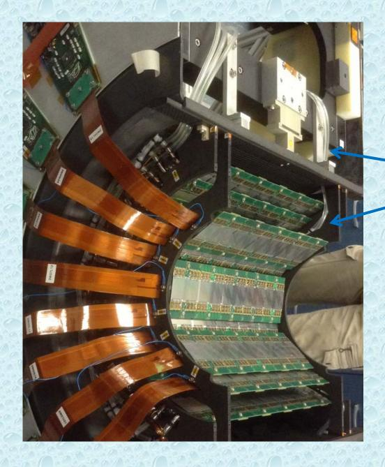
These are the lines shown in the first slide from the inside. As you can see, any water dripping in will drip directly on the strip pixels. These are the lines that feed the inner strip barrel.
