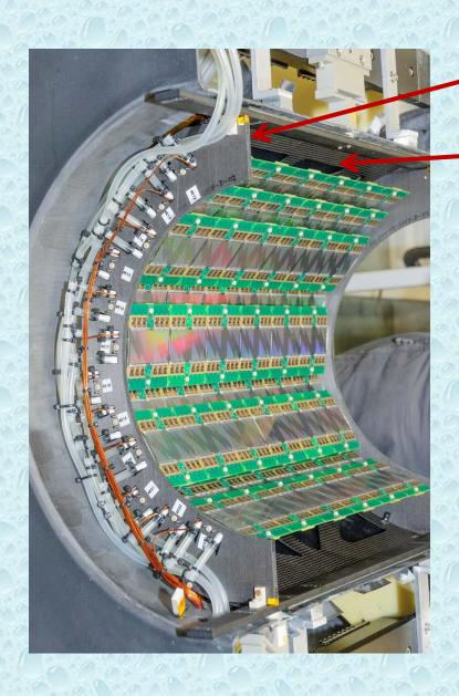
Window Frame seal is behind the carbon frame. If water get in anywhere, it can drip from the edge of the carbon frame onto the back of the Strip Pixels. These are the FVTX supply lines as they enter the enclosure. They are right next to the Strip lines shown in slide 2. They run at the same temperature (below 10C) and will condense water if exposed to air.
