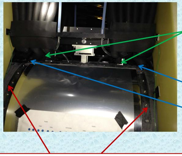
Gap between insulation and detectors must be air tight to prevent condensation. We had water in many areas along the cooling lines once the humidity in the IR went up in June.
