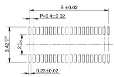
Recommended solder paste thickness: 120  $\mu$ m
