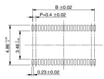
Recommended solder paste thickness: 120  $\mu m$
