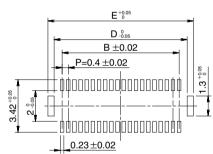
Recommended solder paste thickness: 120  $\mu m$
