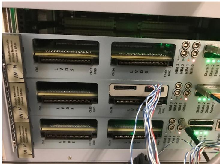
Figure 2: Stack of 3 MOSAIC cards. The additional card in the central MOSAIC is the mezzanine, which is connected to the power board via twisted pair cable.
