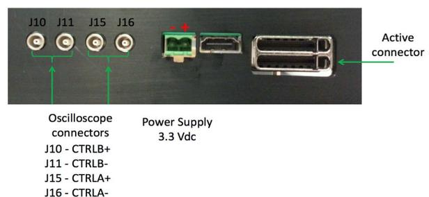
Figure 4: Rear view of the module box with the new adaptor for the DCTRL measurement (left) and pinout (right)
