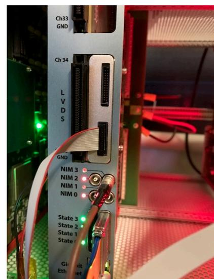
Figure 12: Oscilloscope and MOSAIC connections for DCTRL measurement
