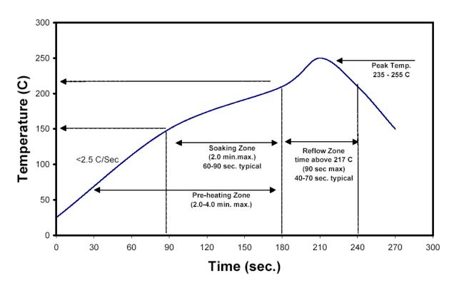
Kester Lead Free Reflow Profile Alloys: Sn96.5/Ag3.0/Cu0.5 and Sn96.5/Ag3.5
