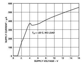
Figure 7. Supply Current vs. Supply Voltage
