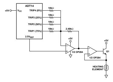
Figure 30. Combination Trip-Point Output
