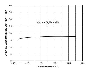
Figure 9. Open-Collector Output Sink Current vs. Temperature
