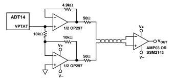
Figure 21. Send the Signal Differentially for Noise Immunity
