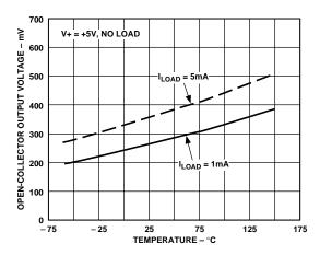
Figure 10. Open-Collector Output Voltage vs. Temperature
