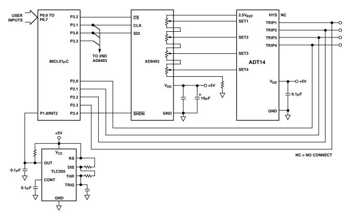
Figure 28. Typical Microcontroller Setup Configuration
