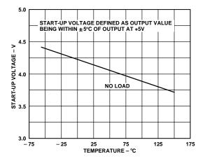
Figure 4. Start-Up Voltage vs. Temperature
