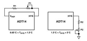
Figure 17. Hysteresis Connections for Miscellaneous Values
