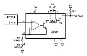
Figure 23. Temperature-to-Frequency Converter
