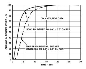
Figure 3. Thermal Response in Stirred Oil Bath
