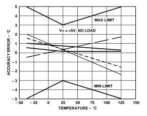
Figure 6. Accuracy Error vs. Temperature, Stirred Oil Bath
