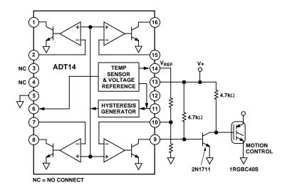
Figure 18c. Driving an IGBT
