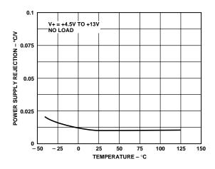
Figure 12. VPTAT Power Supply Rejection vs. Temperature
