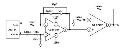
Figure 27. Translating 5 mV/K to 10 mV/°F
