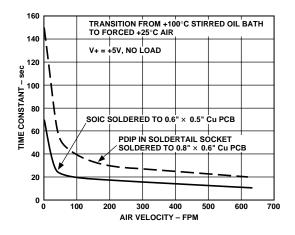
Figure 2. Thermal Time Constant in Forced Air
