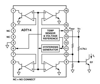
Figure 19a. An External Resistor Minimizes Self-Heating
