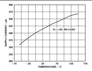
Figure 8. Supply Current vs. Temperature
