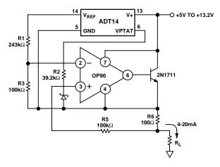
Figure 22. 4 mA to 20 mA Current Loop
