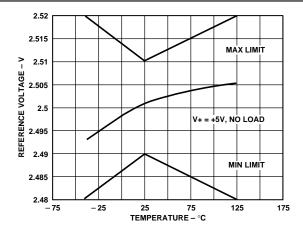
Figure 11. Reference Voltage vs. Temperature
